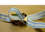
*Adjust the position of the strap around the mold. You need a couple inches of slack.*
